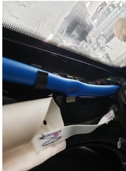
Figure 2. Sunroof drain hose pinched by pillar trim.
