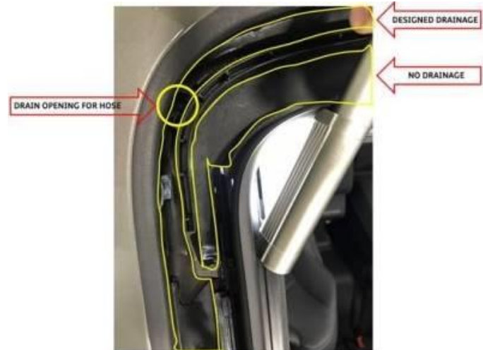
Figure 7. Sunroof water channeling diagram.
