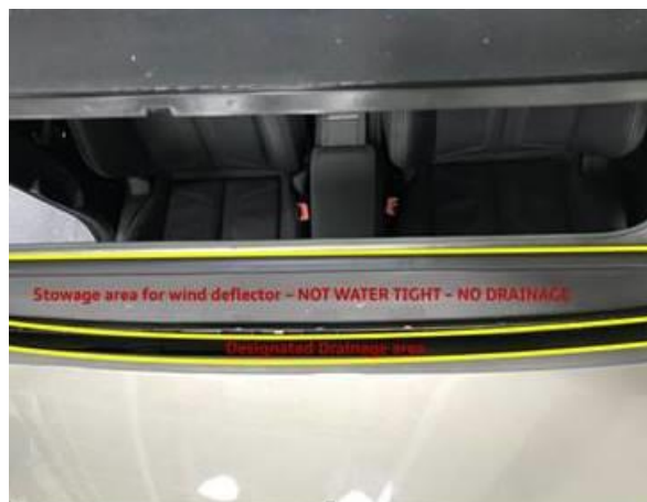
Figure 6. Areas of sunroof opening water elimination capabilities.
