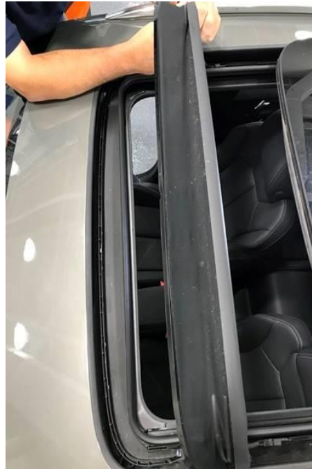
Figure 5. Front sunroof opening with drainage exposed.
