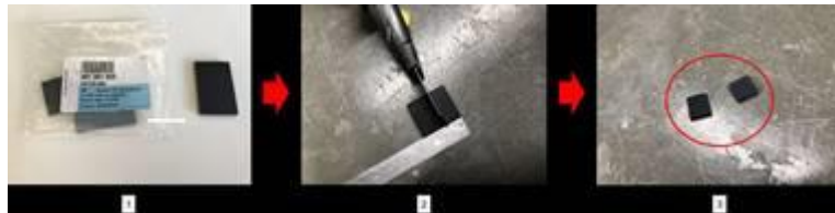
Figure 15. Preparing 2 – 10mm x 10mm pads of 251 201 525 packing.
