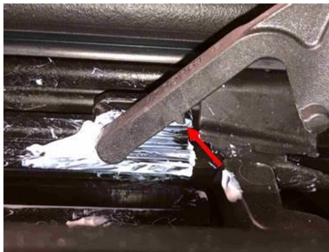
Figure 9. Tabs cast into the redesigned wind deflector.
