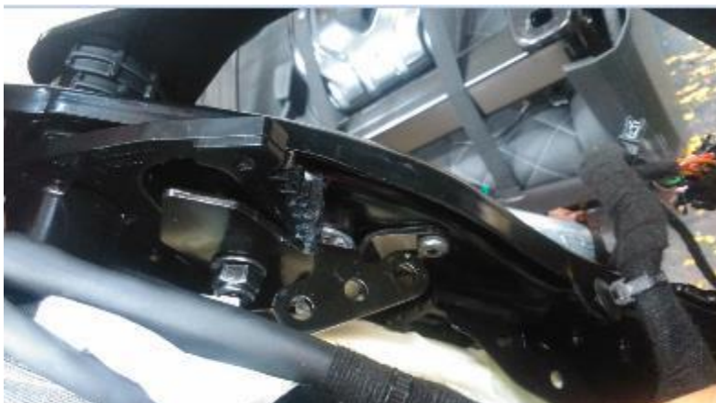
Figure 2. Toothed segment of the seat height adjustment.
