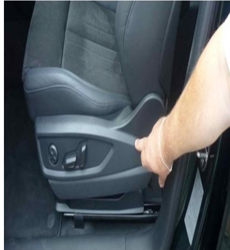
Figure 1. Noise originates from behind the seat frame trim panel near the hinge.
