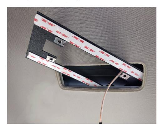
Pamove the backing from the tape strips center the four screw holes acking plate in the headliner opening. Press the plate into place once centered.
