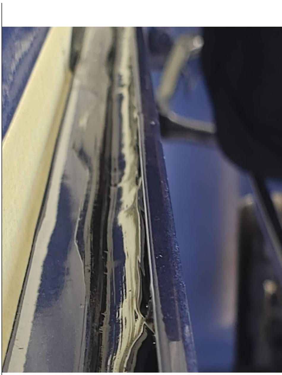
**5. Let the sealant dry according to manufacturer instructions. Sealant should not be visible when looking at the back of the vehicle.**
