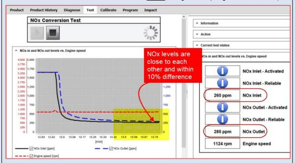
If both NOx sensor ppm levels are **close to each other** at a point during the test as shown in the examples (image) above, then both NOx sensors are good.
