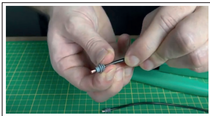
Figure 6 - Sliding the Seal down
