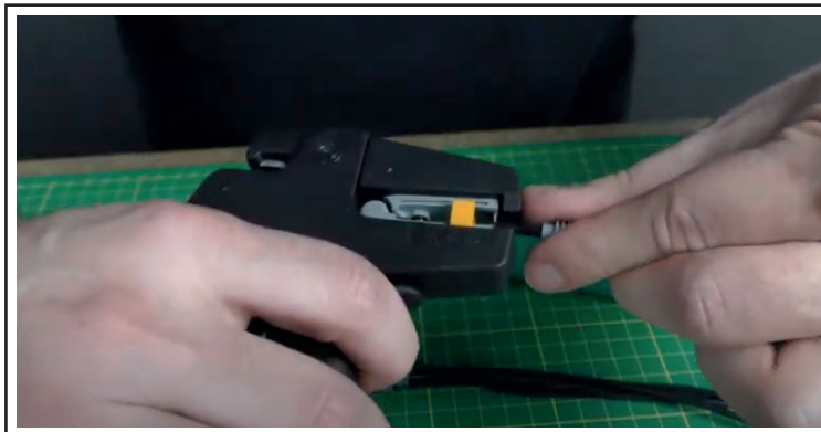
Figure 5 - Stripping of the Wire
