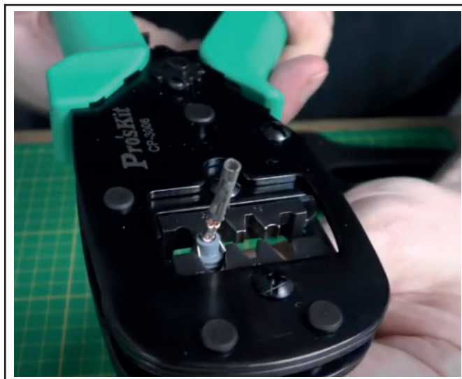
Figure 9 - Crimping the Larger Tab on the Terminal
