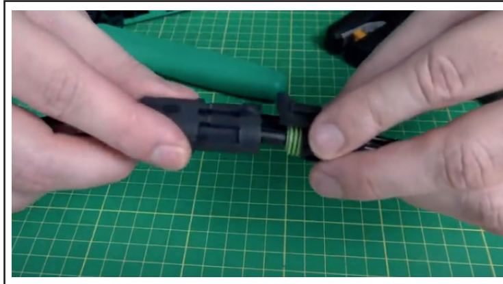
Figure 13 - Assemble the Weather Pack Connector
