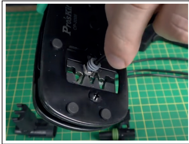
Figure 8 - Crimping the Smaller Tab on the Terminal
