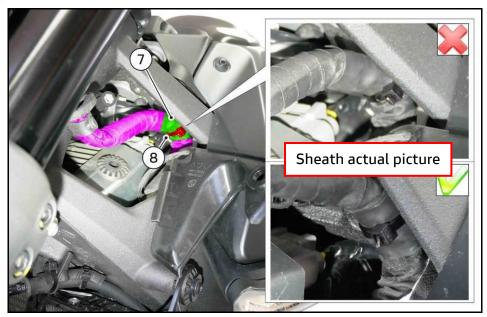
**2 A.** Should the tie be already correctly positioned at the center of the sheath, mark the check with a felt pen (see figure below), then proceed to step 8
