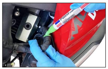
5. Insert the new large self-locking tie (11) inside the seat on frame, aiming it as shown in the figure
