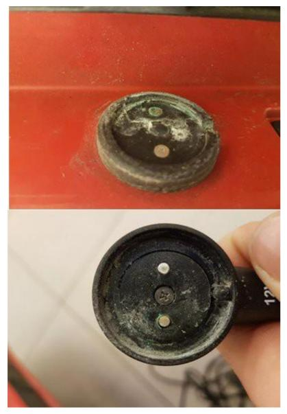
If light corrosion is present, use Autosol metal polish or an equivalent metal polish to remove the corrosion from both the charger socket and the charger lead.
