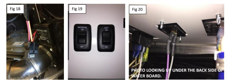
**Correction for Cause #4:MY16-21:** The macerator or hose is plugged and will not empty the tanks. Remove the obstruction in the impeller or the hose.
