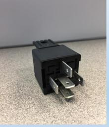
WITH SWITCH <u>ON</u>, TEST FOR 12V B+ AT TERMINALS #30 AND #87. USE ANY GROUND. **Correction for Cause #3:MY16-21:** The macerator switch has failed or wires have lost connection at the switch or the relay in the wet bay. Check wire connections on the relay and switch in water bay board shown in Fig 18-20.
