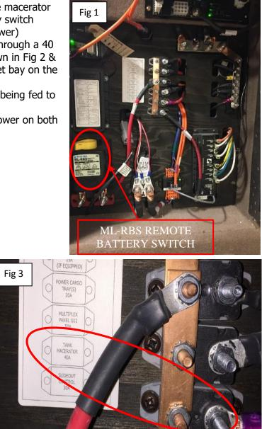
Correction for Cause #1: MY 19 & 20: The breaker for the macerator in MY 19 & 20 is tripped off at the DCD board on the passenger side battery compartment shown in Fig 3 & Fig 4.
