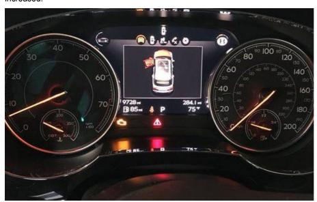
Diagnostic Trouble Code (DTC) 'P218100 - Cooling System Performance' is stored in the Engine Control Module (ECM), the vehicle "warm up" time is longer when compared to other vehicles of the same type.
