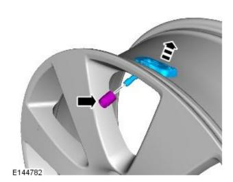
Remove the sensor retaining nut and then remove the tire low pressure sensor and valve assembly.
