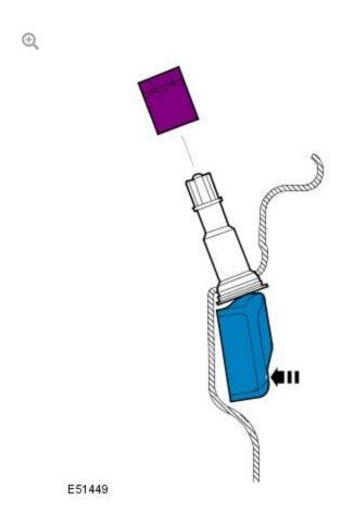
Install the original tire low pressure sensor into the new wheel.
