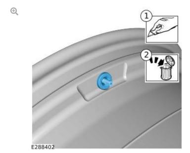
Use a suitable tool to remove the rubber valve.
