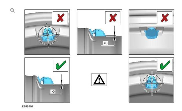
Check if the tire low pressure sensor is installed correctly, as shown in the images with a **GREEN** '\s'. If the sensor assembly is installed incorrectly, as shown in the images with a **RED** 'X', do not try to adjust or rotate the sensor and valve. Remove and install a new rubber valve.
