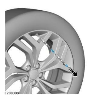
Use a suitable tool to remove the valve cap and the insert. Allow the air to fully escape from the tire before attempting to remove the tire from the wheel.
