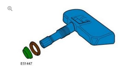
Remove and discard the seal and washer.
