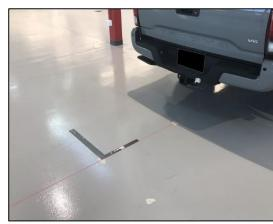
Create a perpendicular crossline that intersects all 3 points (two points created by the square and the vehicle centerline point) and extend the perpendicular line past the target/marker placement point.
