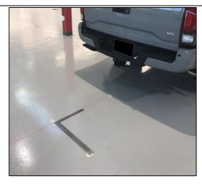
4. Using the square on the **opposite** side, align one leg along the centerline, with the other leg perpendicular to the vehicle centerline. Mark the furthest point out on the square.
