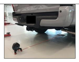
4. Place the laser target from the SST kit (PN 00816-00103) on the **FRONT** vehicle centerline mark.
