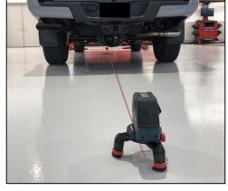
6. Create the perpendicular line using the 90-degree laser.
