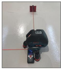
8. Without moving the base, rotate the laser 90 degrees counter-clockwise to extend your perpendicular line towards the opposite target/marker, then repeat Step 7.
