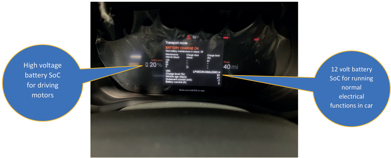
Figure 2. Do not confuse HVB SoC and 12V batt SoC
