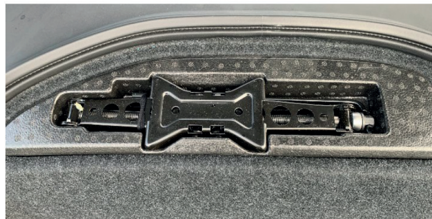
Figure 11. Jack is above toolkit, either package
