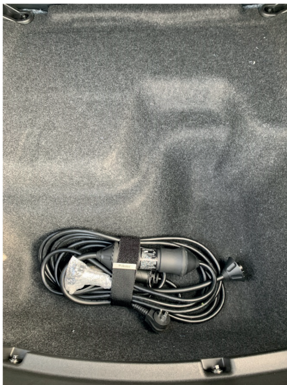
Figure 4. Place charge cable under trunk floor. Wrap with velcro strap if it has one
