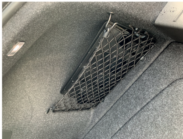
Figure 3. Placement of front license plate frame and hardware in right rear cargo area if the customer's state of registration does not require a front plate.
