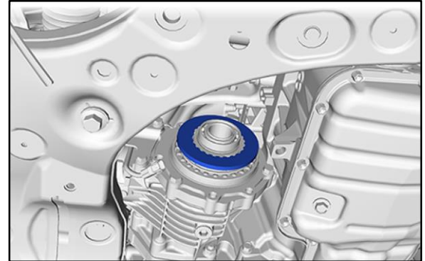
Figure 13. Armature Plate Installed
