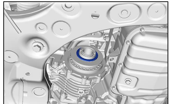
Figure 24. Thrust Roller Bearing Installed
