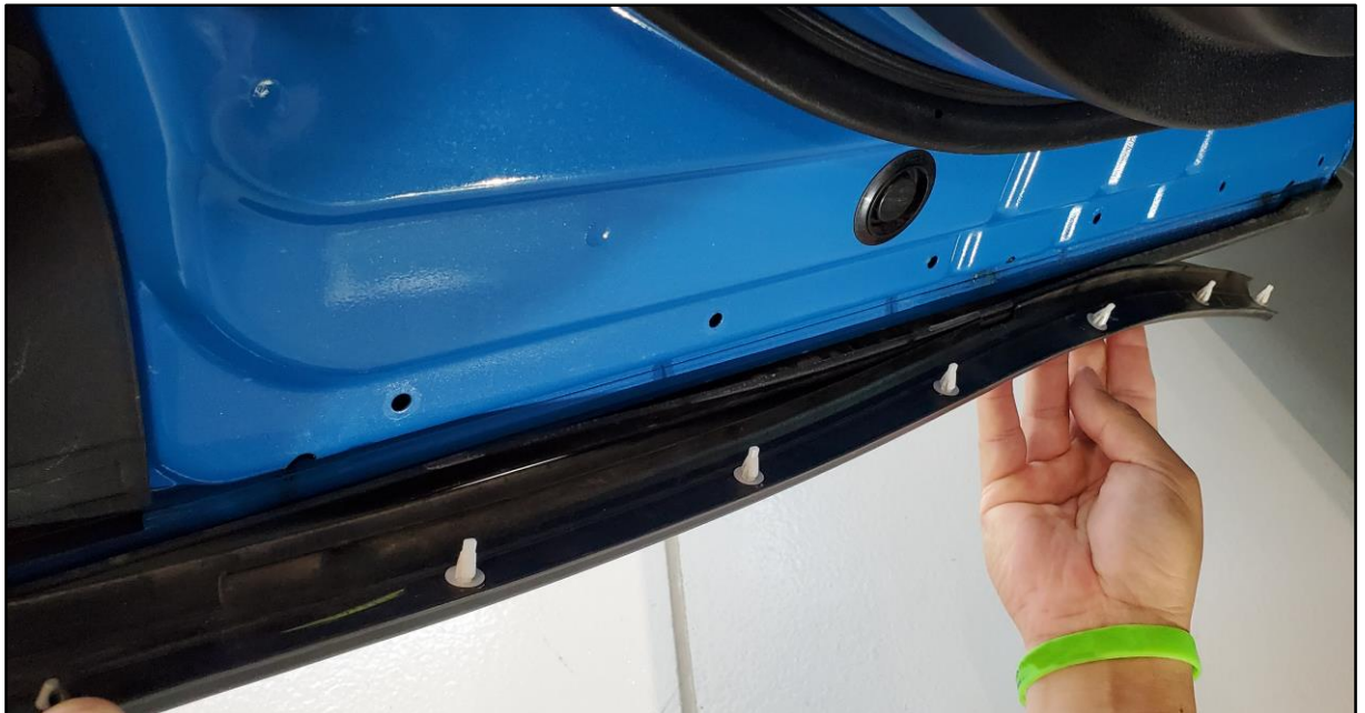
Figure 12. Reinstalling Weatherstrip Moulding to Door
