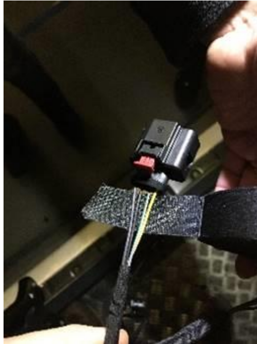
Figure 2. Harness is wrapped using textile tape 105 920 02.
