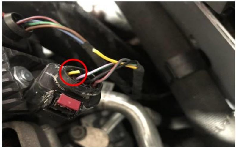
Figure 1. Wire is broken at G31 sensor.
