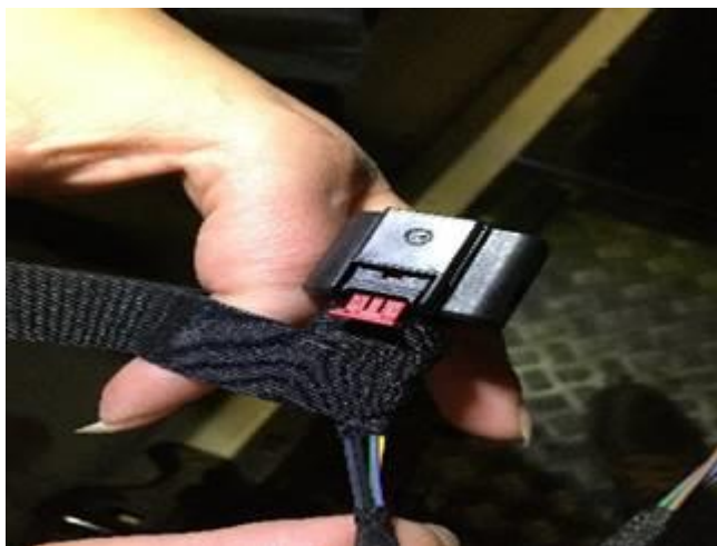
Figure 4. Wrapping the connector base part 2.
