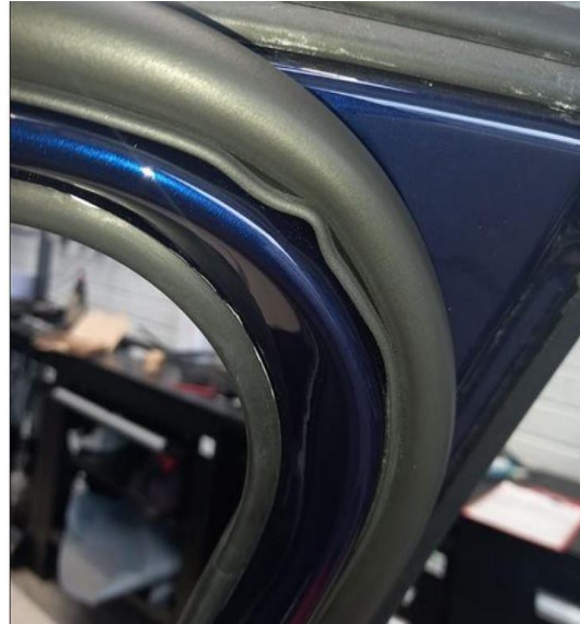
Figure 1. The outer door seal detached from the door.
