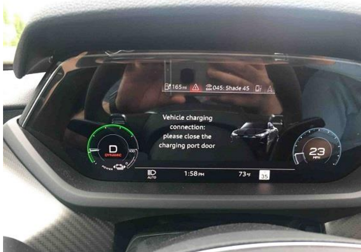
Figure 1. DIS message incorrectly requesting to close the charging port door.
