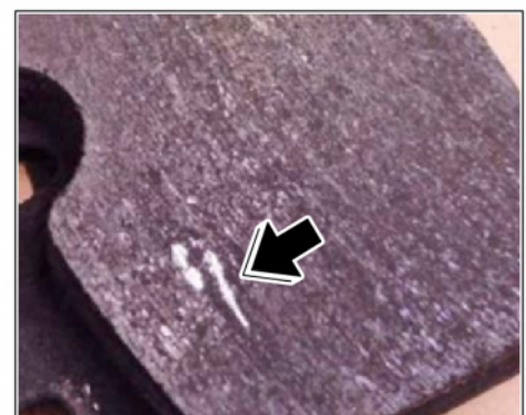
Particles of dirt on brake pad
