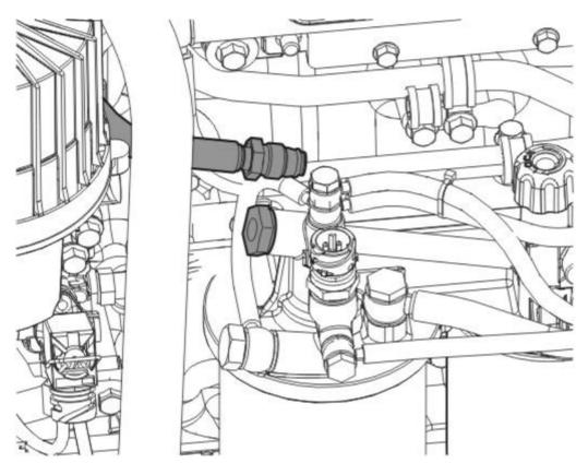
Remove cylinder head fuel return line hose connection at engine fuel filter housing and install plug from kit with new copper sealing washer.
