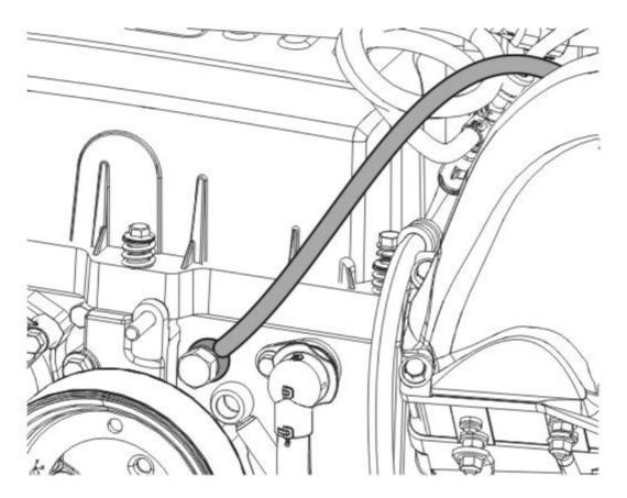
Note: Clean the connection points before installing the line.
