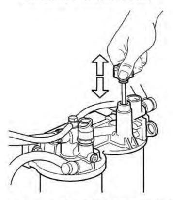
The 1/4 turn lock hand primer pump is not a source for air in the fuel, but it will block off fuel supply to primary filter and engine will eventually run the primary filter dry of fuel if left in the unlocked position.
