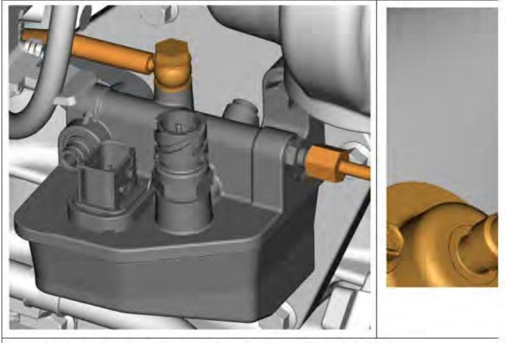
Tighten all Integrated Aftertreatment Hydrocarbon Dosing System fuel line fittings to 15 Nm (135 in-lb)
