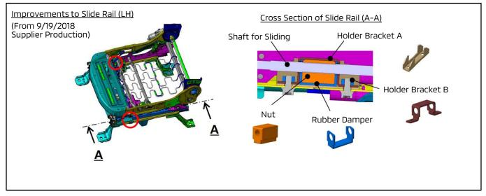
The clearance of the bearing plate hole size has also been changed in production at the supplier starting May 10, 2021. Refer to the VINs listed in Affected Vehicles.
