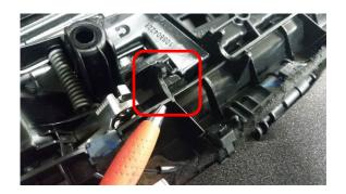
**Cause:** The investigations carried out have shown that this breakage can occur when removing the door panel.
