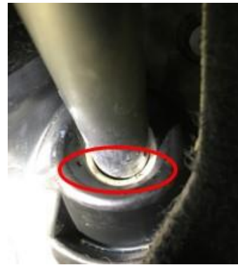
Figure 1. Poor sealing on the intermediate shaft.
