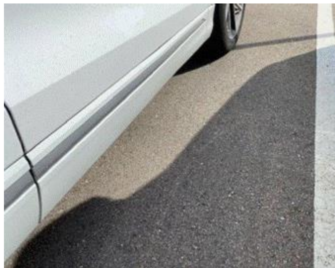
Figure 1. Visible gap present between the front door trim cover and the outer door panel.
