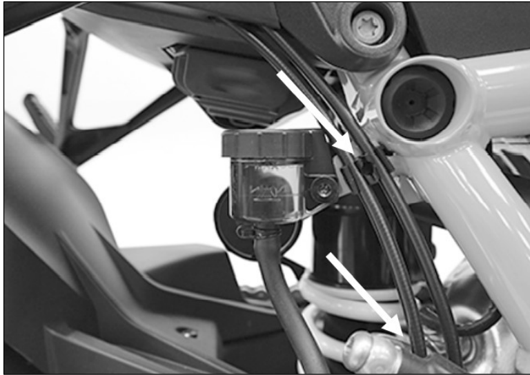
Fig. 2 – Cables in the area of the brake line
