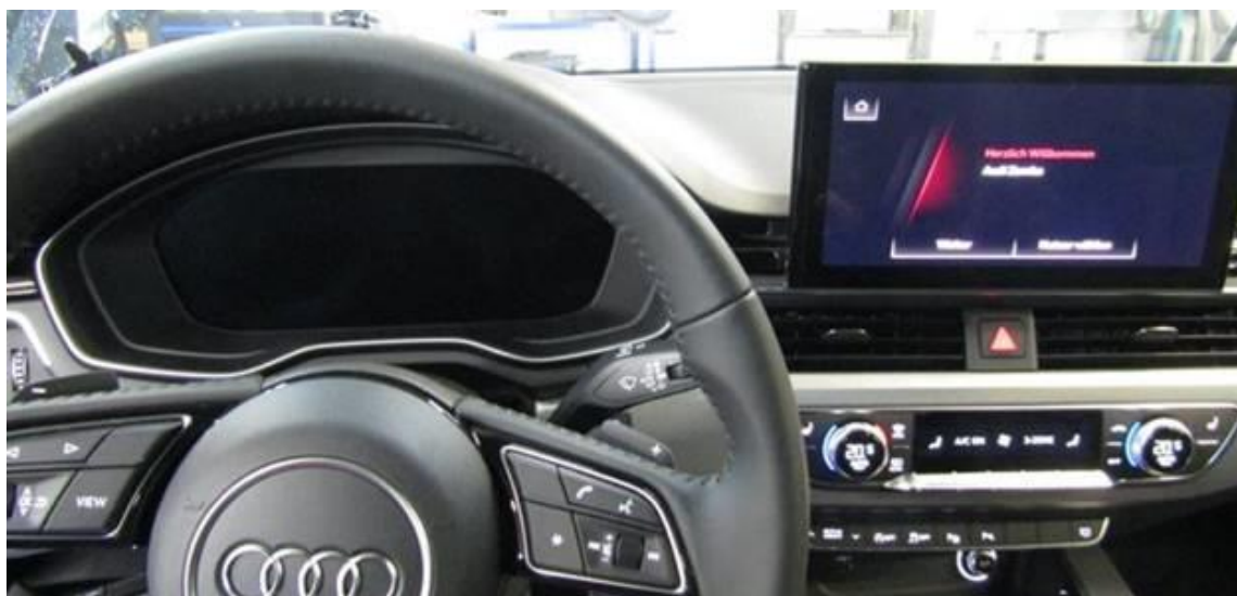
Figure 1. Audi virtual cockpit does not start-up; the screen remains blank (example).
