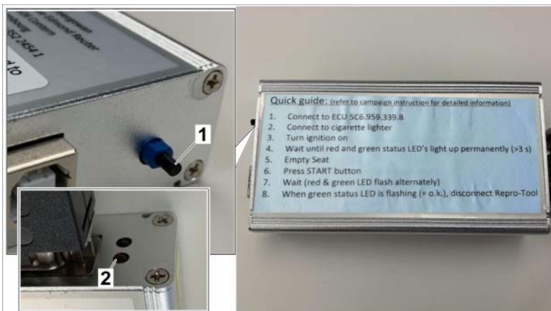
Re-programming control unit
