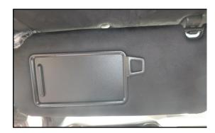
2. Pull down on the sun visor to inspect if the retainer is broken (approx. 5 lbf).
