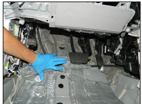
Figure 6. Driver Side Dash Panel Insulator Assembly Inspection
