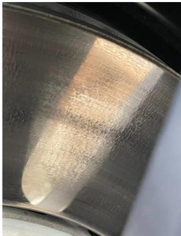
Figure 1. Brake disc surface cracks.
