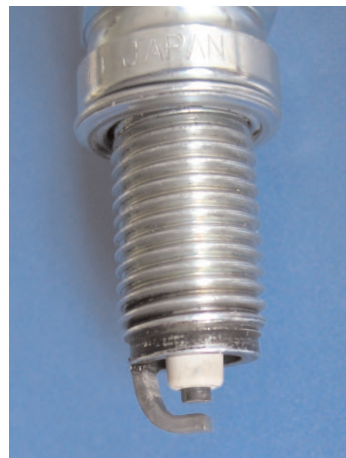
Spark plug in good condition
