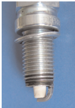
Insulator broken and slipped down onto ground electrode
