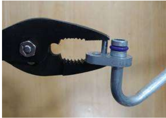
Figure 16. Installation of rear refrigerant line dowel pin.
