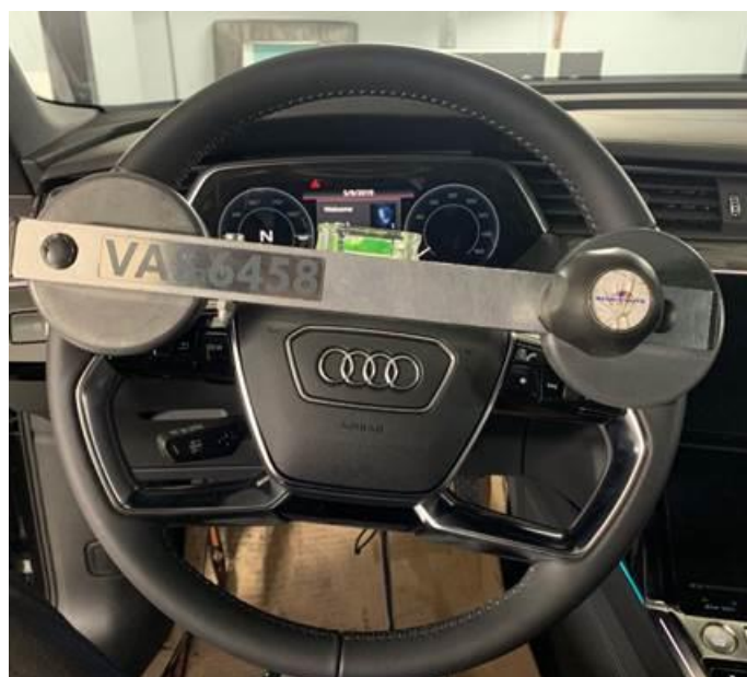
Figure 1. VAS 6458 installed with steering wheel off-center.
