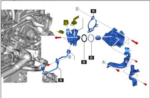
· Gasket and O-rings for water pipes and cylinder head gasket
