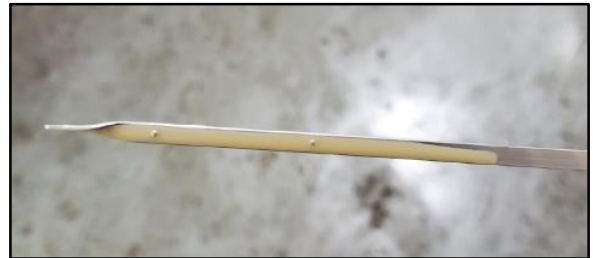
Figure 2. Engine Oil (Milky/Discolored)
