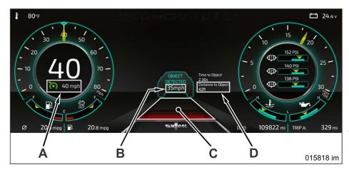
A Set cruising speed B Speed of forward vehicle C Set following distance D Following distance
