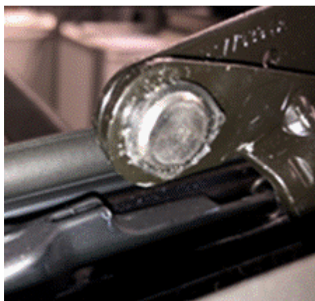
Figure 5. Water guidance washer on the front frame mechanism pivot.
