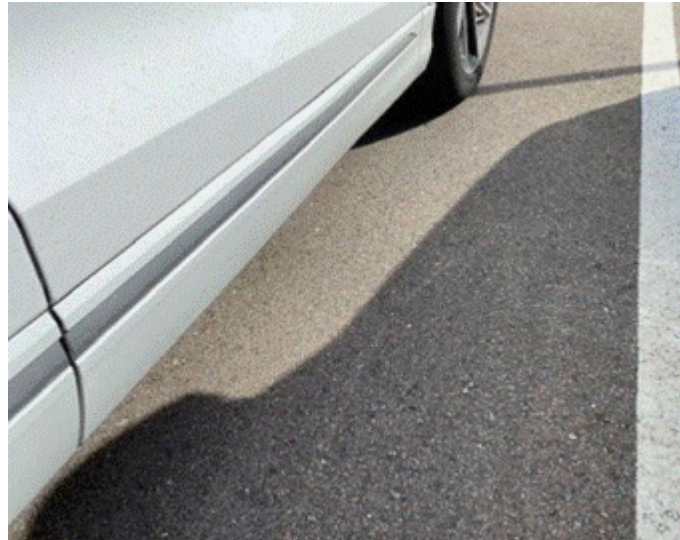
Figure 1. A visible gap is present between the front door trim cover and the outer door panel.
