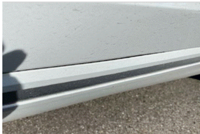
Figure 2. A closer view of the gap, which is present between the front door trim cover and the outer door panel.
