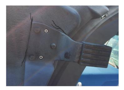
• If the cracks have spread to the point that the guide and backing plate are missing support along multiple edges or is completely broken out, the hood will need to be replaced.
