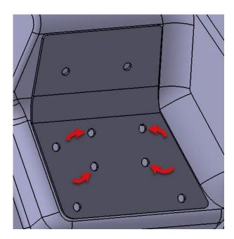
**4.1.4.** Prior to tightening the bolts or making any marks, ensure the backing plate is in proper contact (flush) with all three of the surfaces it will mount to as shown below:
