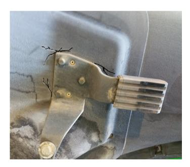
• For a hood guide that has broken away from the hood, the hood may be reused as long as the hole is not much bigger than the old guide bracket. The new plates and guide will attach around the damage:
