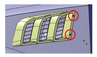
**3.1.2.** Pull the rear of the grille away from the hood, then slide the grille toward the cab to disengage the front mounting tabs.
