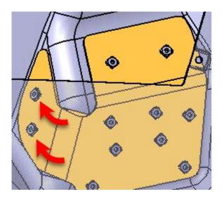
**4.1.7.** Unbolt and remove the front and back plates
