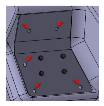
**4.1.6.** On the backing plate, mark the two holes indicated below.
