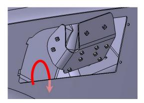
**4.1.3.** Put the new front plate into position on the underside of the hood. Temporarily bolt the front plate the back plate using the four center holes indicated below:
