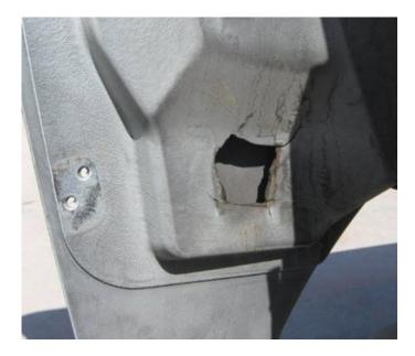
• If there is any other damage to either side beyond what can reasonably be repaired with the procedure below, replacement of the hood is recommended.
