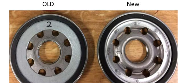
Volvo 21879886 Shallow Groovewill not fit on the US2017 fuel filter housing
