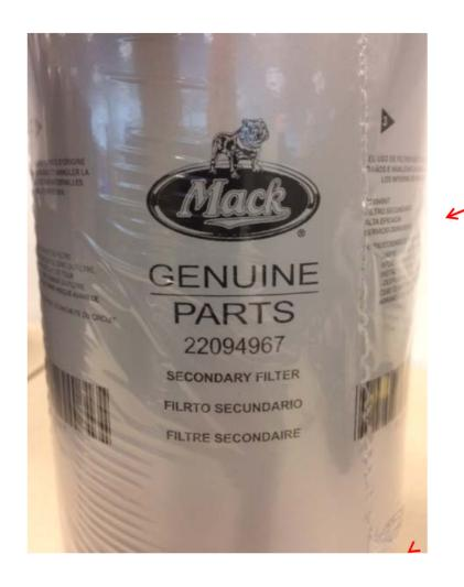
Large capacity Filter media 4 Micron rating
