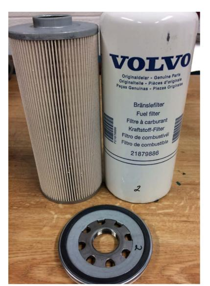
Shallow Groove- Does Not fit on the 2017 fuel filter housing
