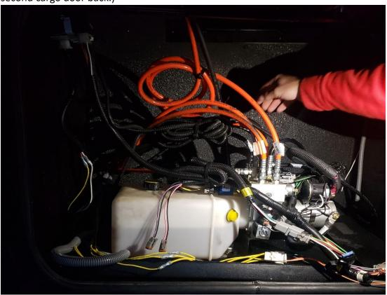
3. Locate the orange and black hydraulic lines labeled "BED SLIDE." (This will be the fourth orange line and the fourth black line.)
