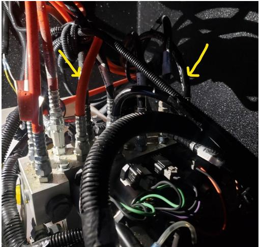
4. Using the 11/16" wrench, swap these lines. (Once the fitting is loose and before you remove the line from the connection point, wrap the rag around the connection point, and then remove the line. This will help contain the remaining fluid to a confined area.)
