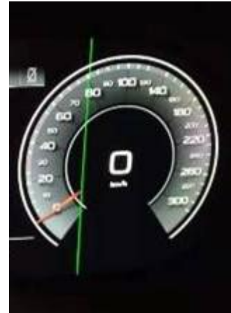
Figure 1. The vertical line through the instrument cluster display.
