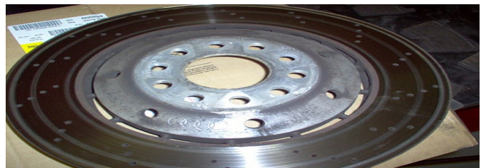
Figure 1. Disc covered with rust.
