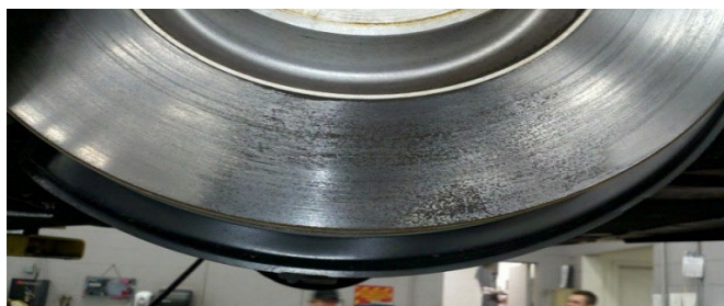
Figure 5. Brake pad material has transferred to the discs.
