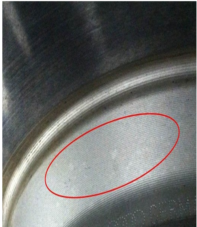
Figure 3. Discoloration on the brake disc due to chemical contamination from the cleaner that was sprayed directly onto the disc.
