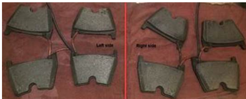
Figure 11. Example of pads without adhesive (mark position for reinstallation if not replaced).
