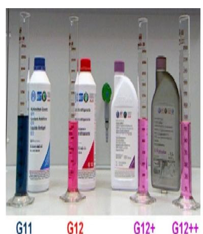
Figure 1. The color of each type of engine coolant. G11 (green-blue), G12 (red), G12+, G12++, G12evo, and G13 (purple).
