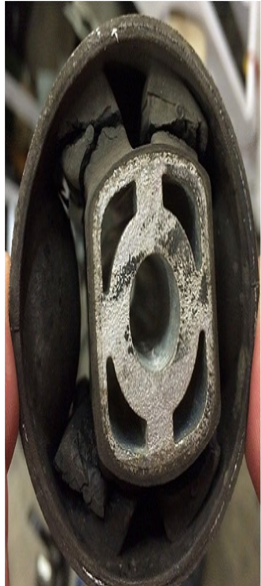
Figure 8. Damaged suspension bushing.
