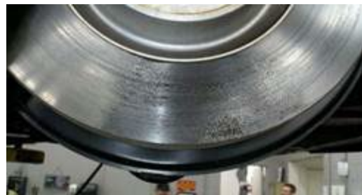
Figure 5. Pad marks on the brake disc.
