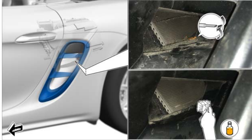
Cleaning air duct
