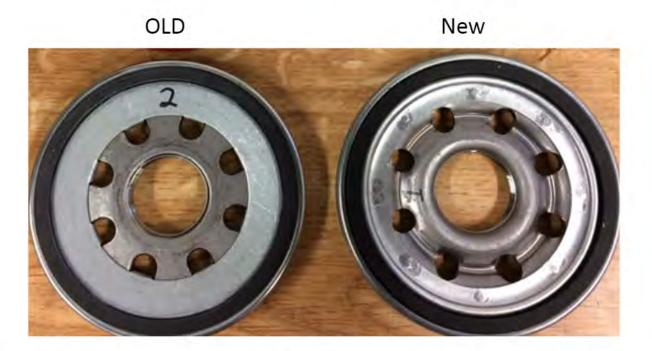
Volvo 21879886 Shallow Groovewill not fit on the US2017 fuel filter housing
