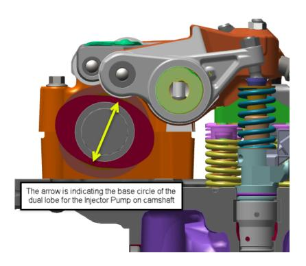
If an injector lobe rotates on the camshaft, the rotation is normally by 60 degrees. It takes approximately 15 degrees of rotation before potentially causing the faults codes listed previously or a fault for a pumping injector during the Common Rail Fuel System Test.
