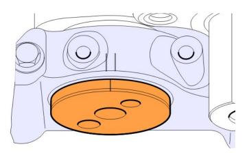
**2.** Once the timing marks are aligned for a specific Injector Pump, verify the injector rocker roller is on the base circle of the injector Live UI efer to the illustration below.
