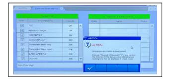
f. Confirm that the erasing and checks have been completed and that no DTCs were detected.
