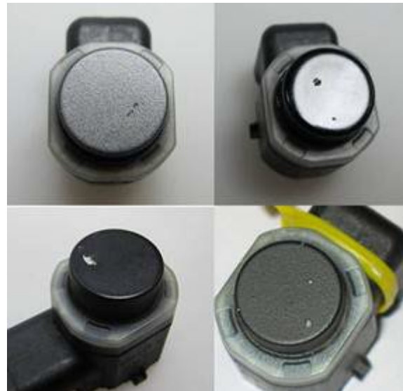
Figure 3. Stone chips causing sensor failure.
