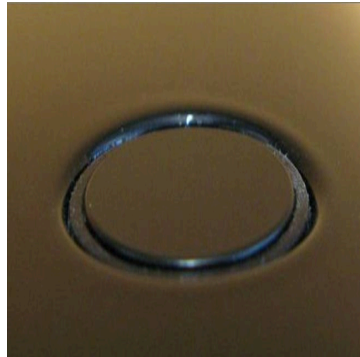
Figure 10. A correctly installed parking aid sensor.
